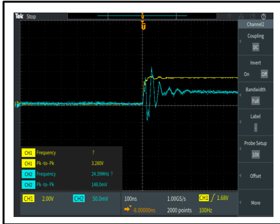
The Switching Rise Time is 200 ns @+25°C
