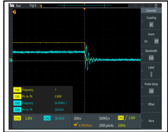
The Switching Fall Time is 200 ns @+25°C
