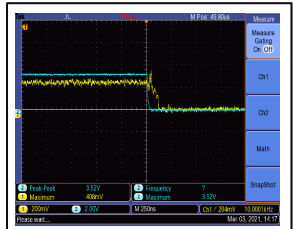
The Switching Fall Time is 150 ns @+25°C
