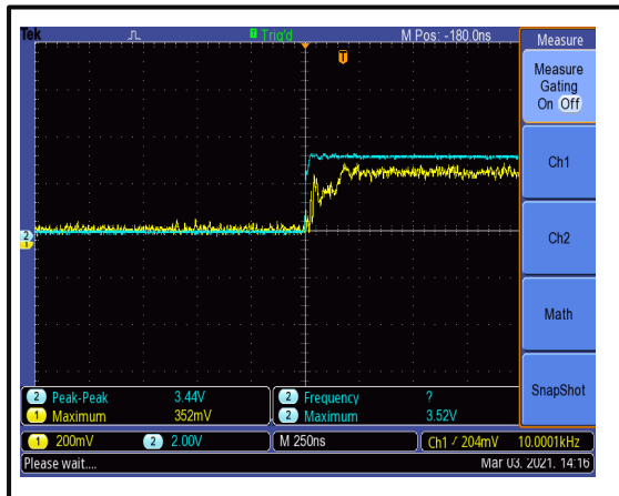
The Switching Rise Time is 200 ns @+25°C
