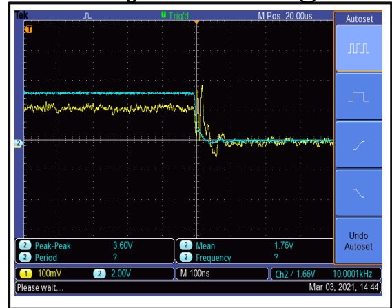
The Switching Fall Time is 50 ns @+25°C
