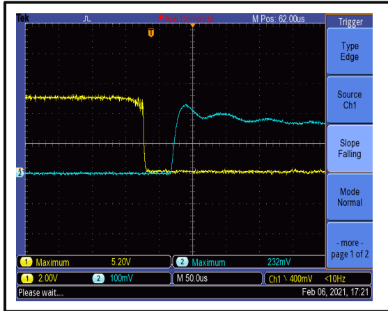
The TDD Enable Time is 50 us @+25°C
