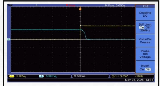
The Drains Closure Time is 200 us
