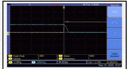
The Drains Closure Time is 150 us
