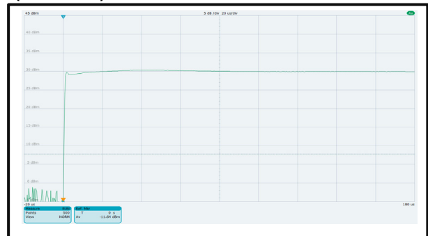
Blanking RF on timing: 40dBm Output Power (20 us/div)
