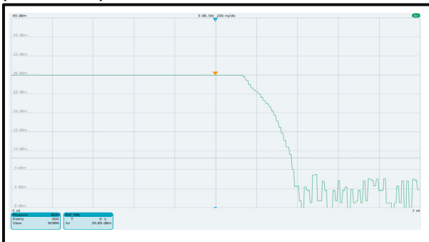
Blanking RF off timing: 40dBm Output Power (200 ns/div)
