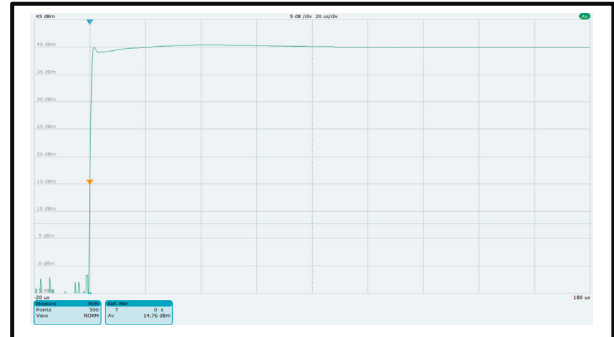
Blanking RF on timing: 40dBm Output Power (20 us/div)
