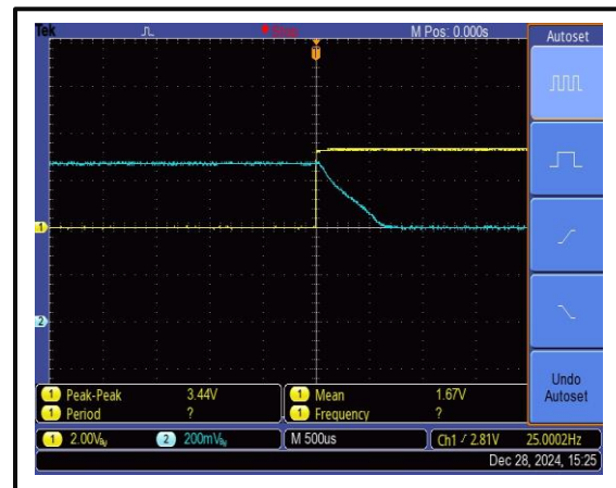
The Drains Closure Time is 600 us @+25°C
