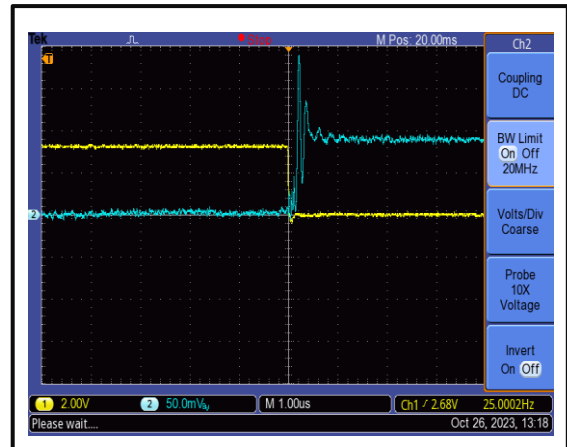
The RF Switch On Time is 600 ns @+25°C
