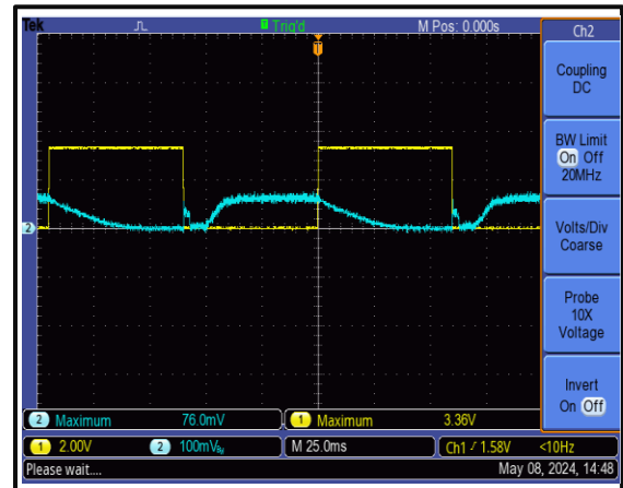
The Drains Open Time is 25 ms @+25°C
