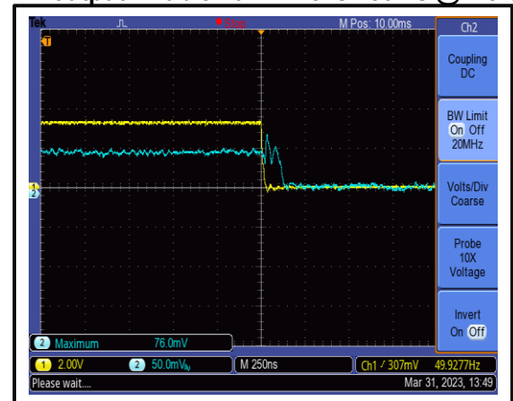
RF output-Enable Fall Time is 150 ns @+25°C
